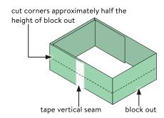
Make cuts in each of the four corners approximately half the height of the Block Out. Remove formed Block Out membrane form, flip over and replace on Block Out spreading flaps to horizontal position. Tape all flaps securely with Barrier-Bac White Bond Tape.
