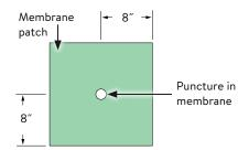
2 Cover damaged portion with membrane patch and secure all patch seams with Barrier-Bac White Bond Tape.
