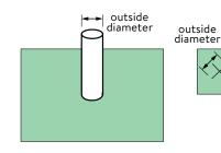
Push the patch to the bottom of the penetration.
