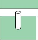
Measure a piece of Barrier-Bac Vapor Barrier membrane 18 inches in width and twice (two times) the circumference of the pipe.
