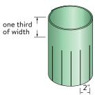
Open boot and wrap snugly around pipe, 6 spreading cuts around base so strips lay horizontal to base.
